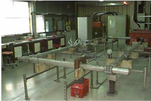
Temperature rise test up to 10kA
